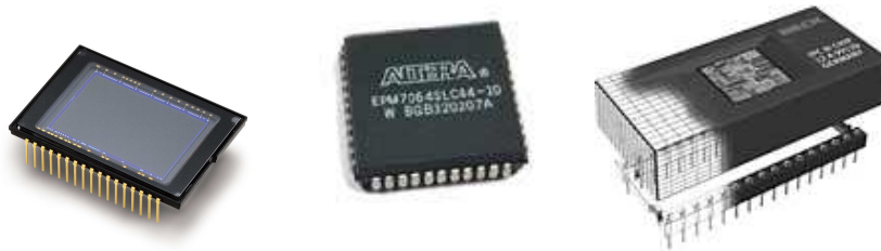
Figure 13: CCD, FPGA chip and embedded computer chips (www.hwwtech.com and www.beck-ipc.com)
